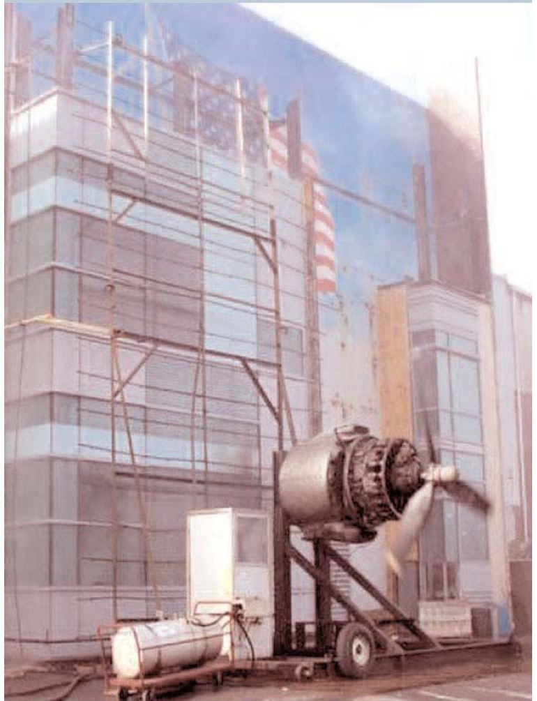
Figure 11. AAMA Dynamic Water Test
